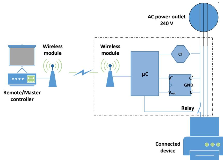
Figure 3: Conceptual design of the smart socket
