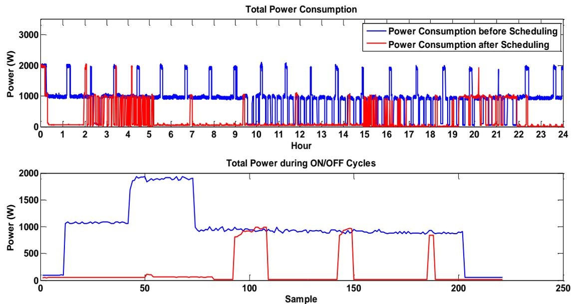
Figure 50: Power consumption trend of all appliances before and after the application of the energy management process
