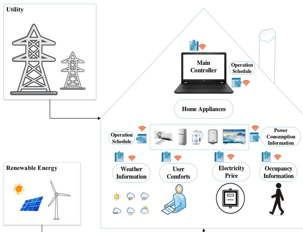
Figure 1: Main components of the HEM system
