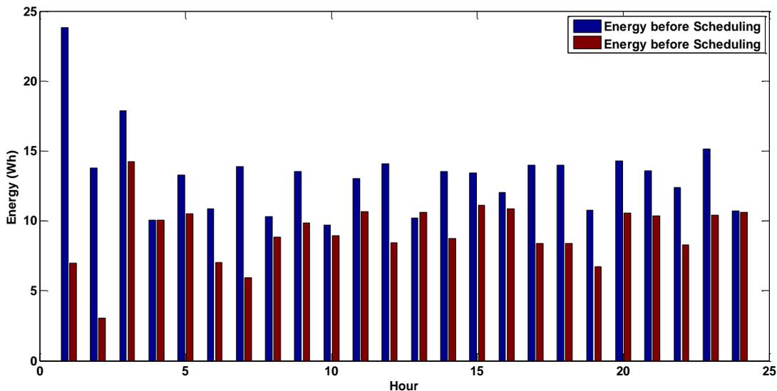
a) Energy consumption trends of the refrigerator before and after the application of the management process
