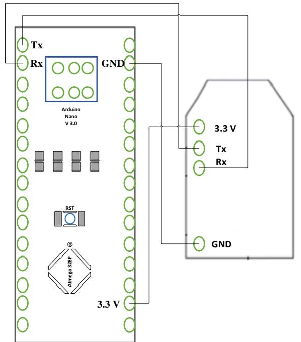
Figure 7: XBee and Arduino interface
