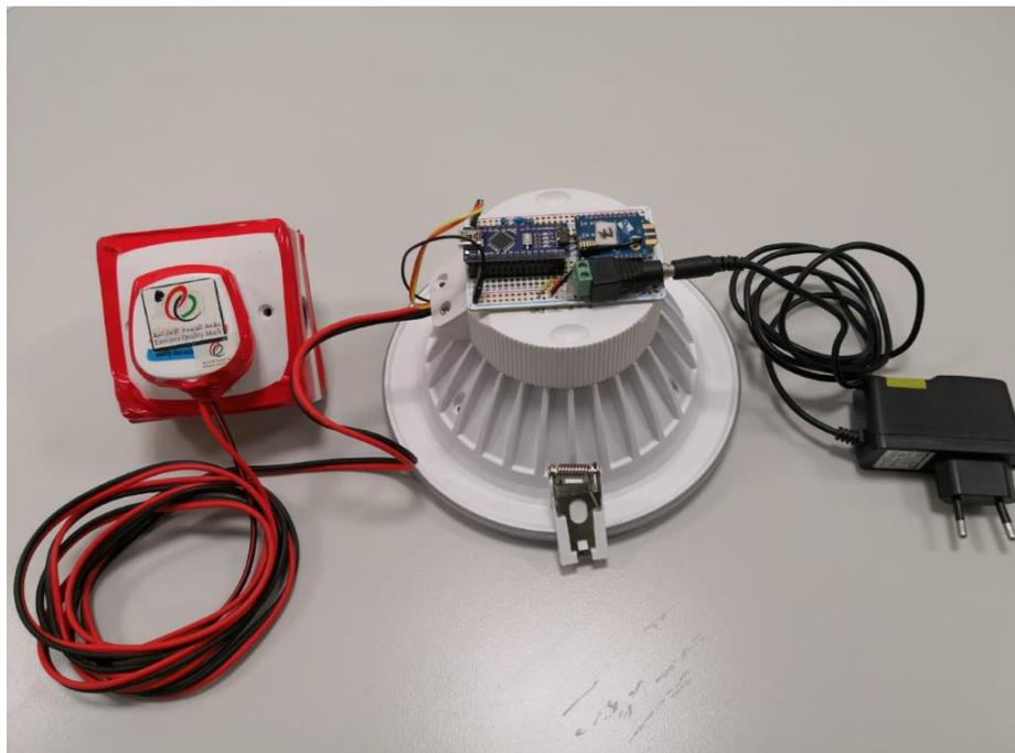
Figure 28: LED energy management experimental setup
