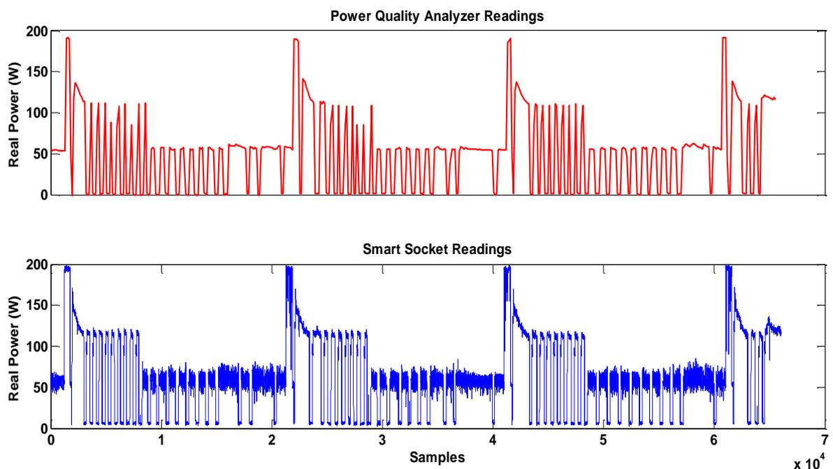
Figure 34: Power consumption trend of refrigerator as monitored by smart socket and PQA
