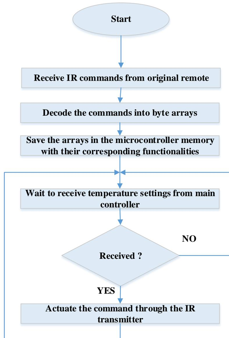
Figure 14: Working principle of the Zigbee-connected remote
