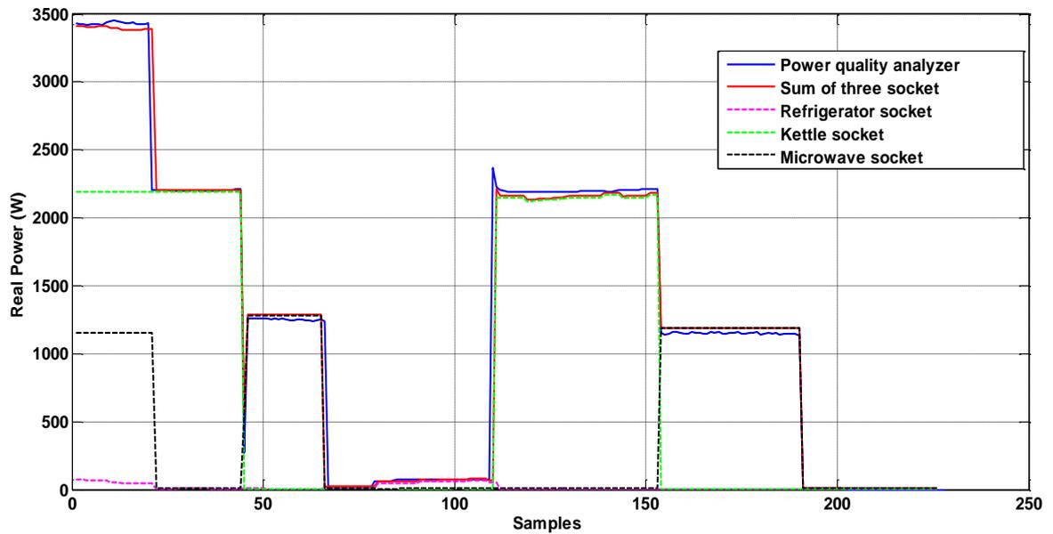
Figure 39: Comparison of power consumption trends of home appliances measured by smart sockets and PQA
