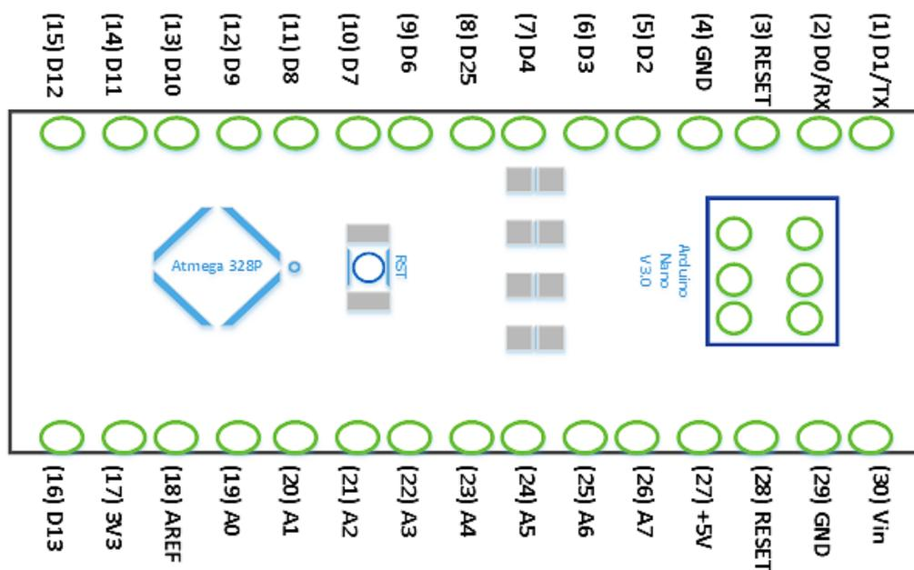
Figure 5: Arduino Nano with pin specifications
