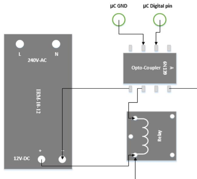
Figure 6: Power supply and relay
