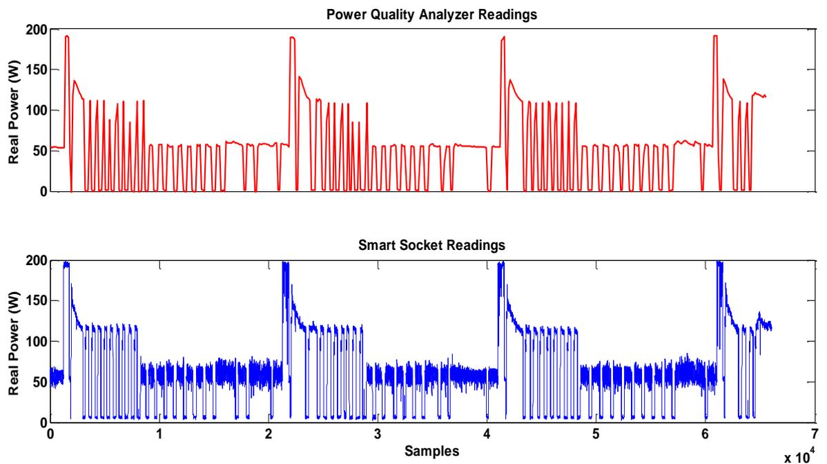
Figure 34: Power consumption trend of refrigerator as monitored by smart socket and PQA
