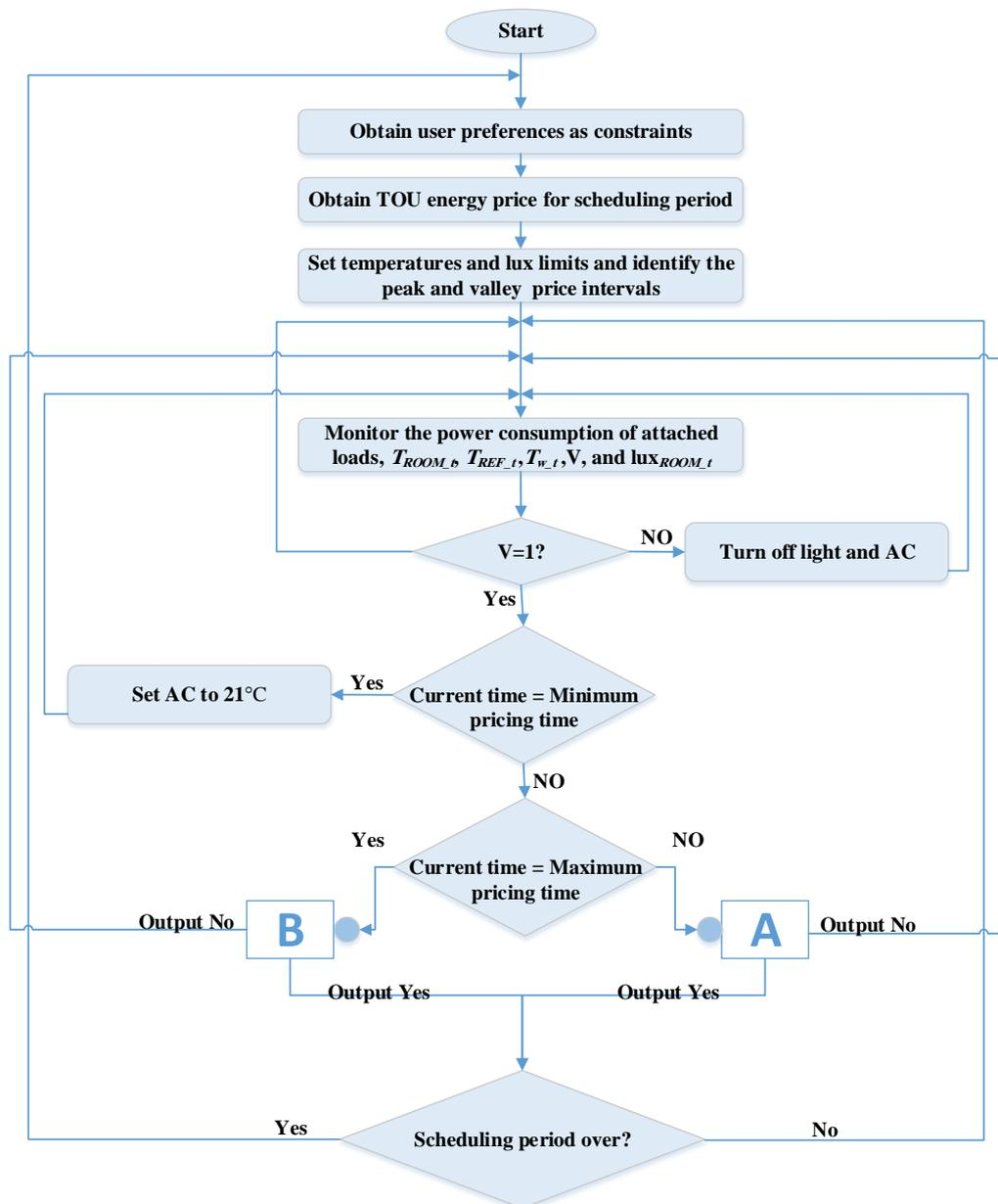
Figure 31: Details of the energy management algorithm
