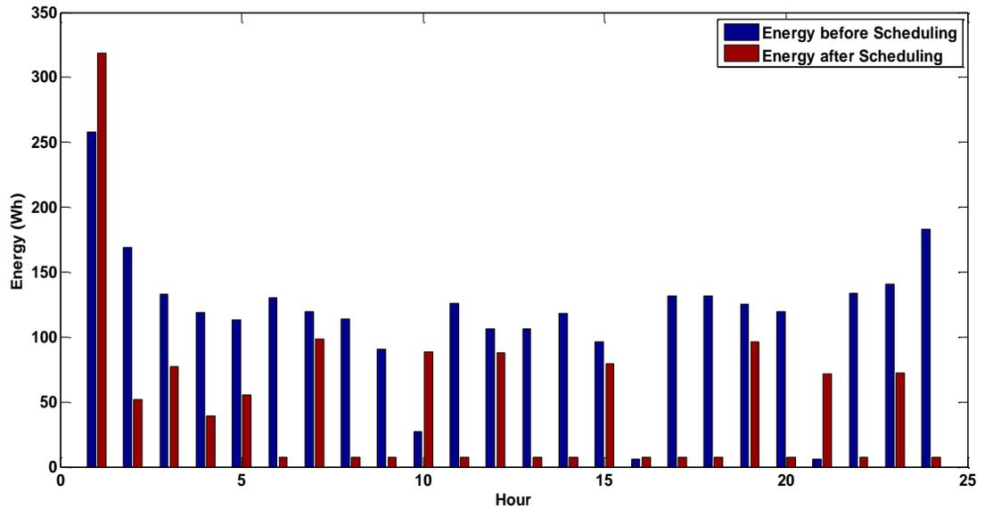
a) Energy consumption trends of the heater before and after the application of the management process
