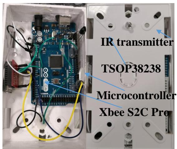
Figure 13: Zigbee-connected IR learner remote controller
