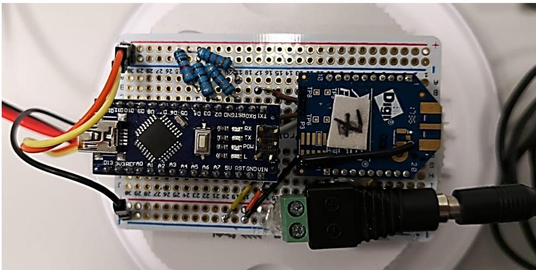
Figure 12: LED light dimming circuit
