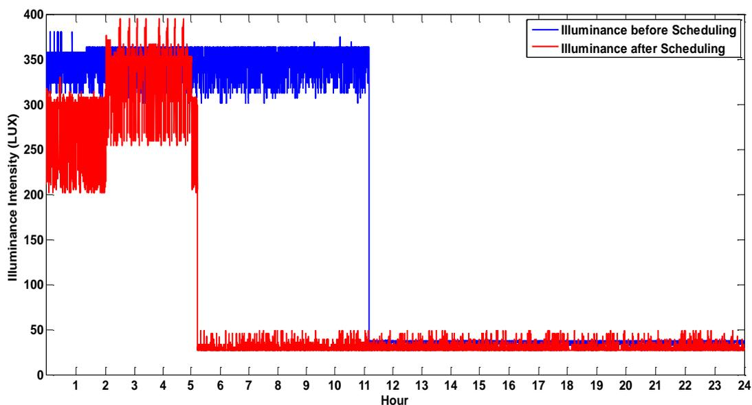
b) Illuminance variations before and after the energy algorithm is applied on the LED light
