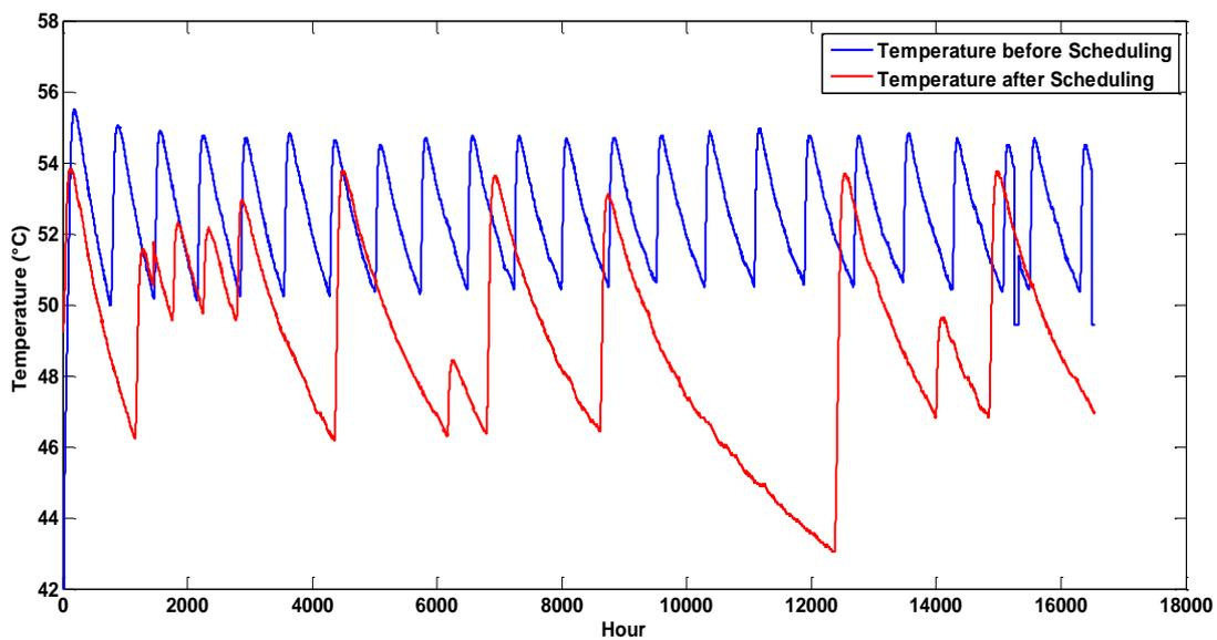
b) Water temperature variation of the heater before and after the application of the scheduling
