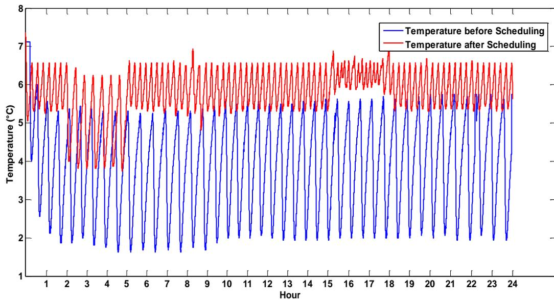
b) Refrigerator inside temperature variation before and after the application of the energy management process
