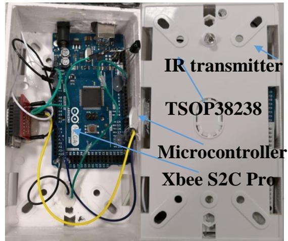
Figure 13: Zigbee-connected IR learner remote controller
