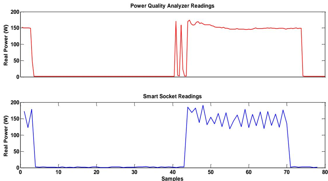
Figure 36: Power consumption trend of electric blender as monitored by smart socket and PQA
