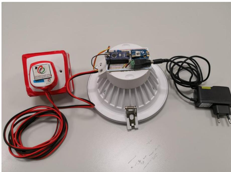
Figure 28: LED energy management experimental setup
