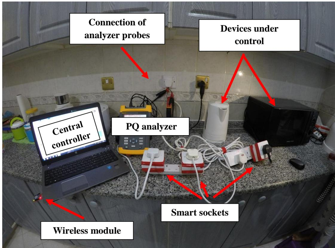
Figure 19: Setup for Experiment 3
