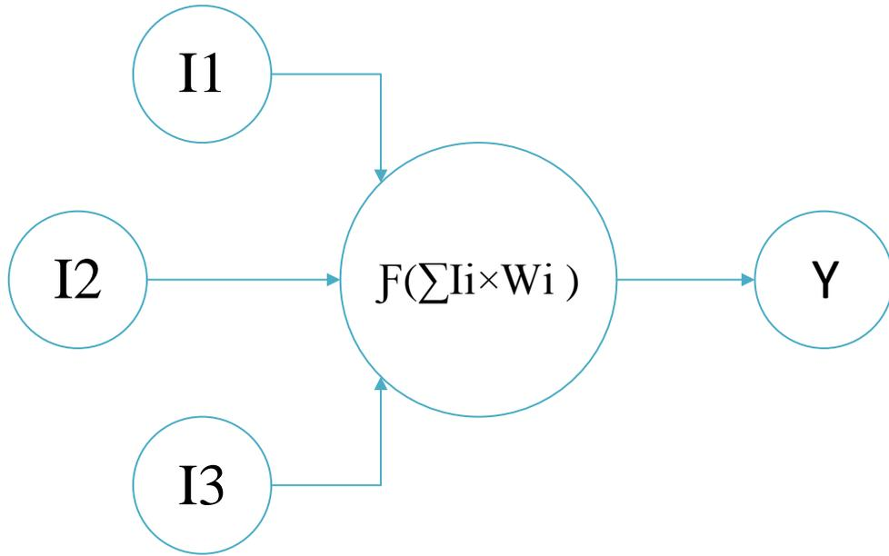
Figure 20: Structure of a single neuron
