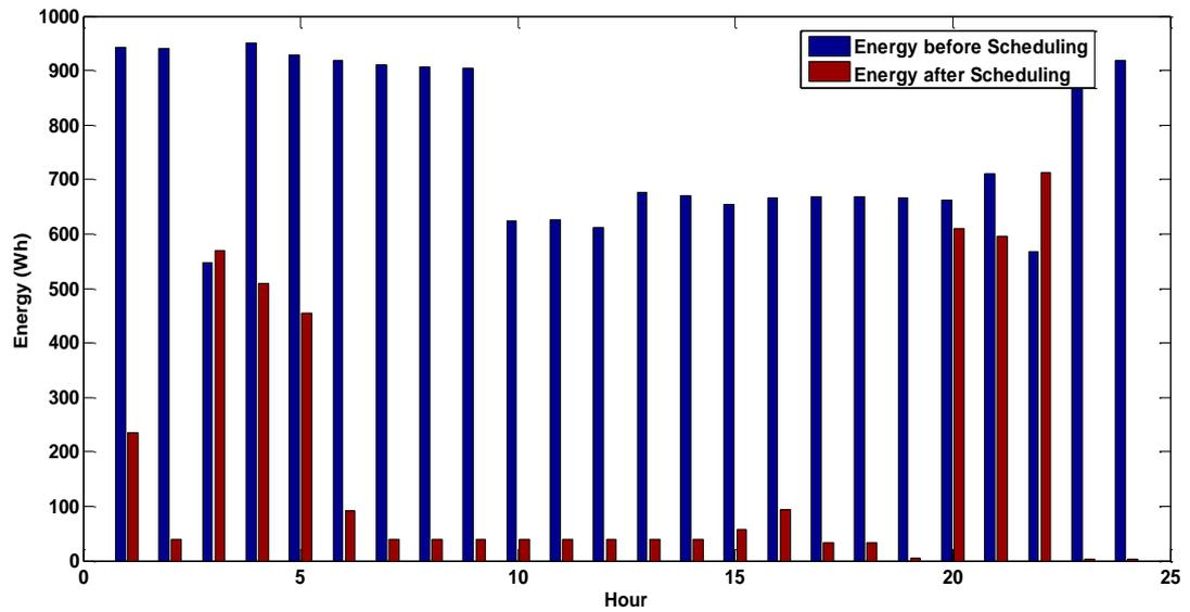
a) Energy consumption trends of the AC before and after the application of the management process
