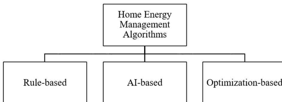
Figure 2: HEM algorithm categories based on the energy reduction technique performed
