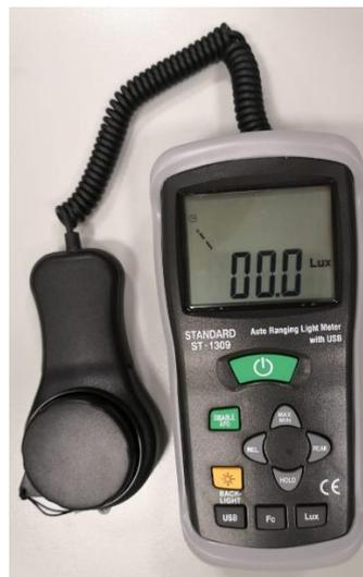
Figure 9: ST-1309 commercial lux meter
