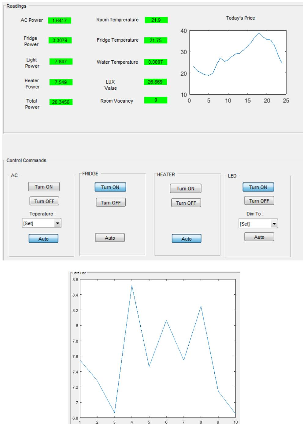
Figure 16: Graphical user interface of the proposed energy management system
