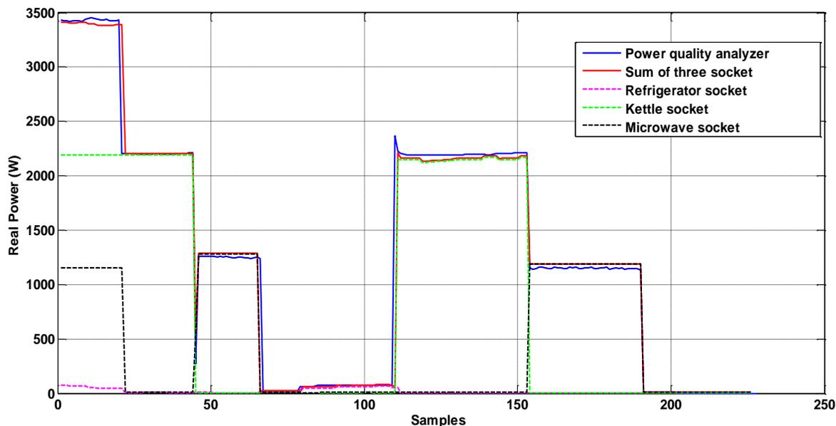
Figure 39: Comparison of power consumption trends of home appliances measured by smart sockets and PQA
