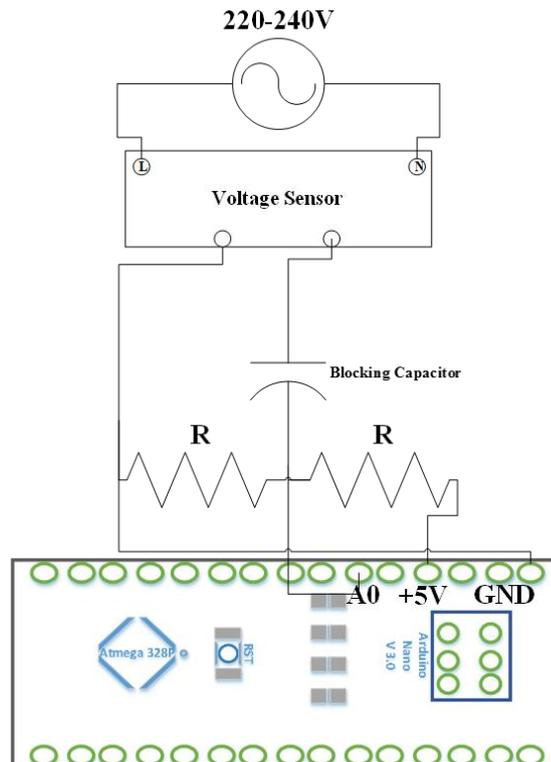
Figure 8: DC offset circuit and voltage sensor connection to the microcontroller
