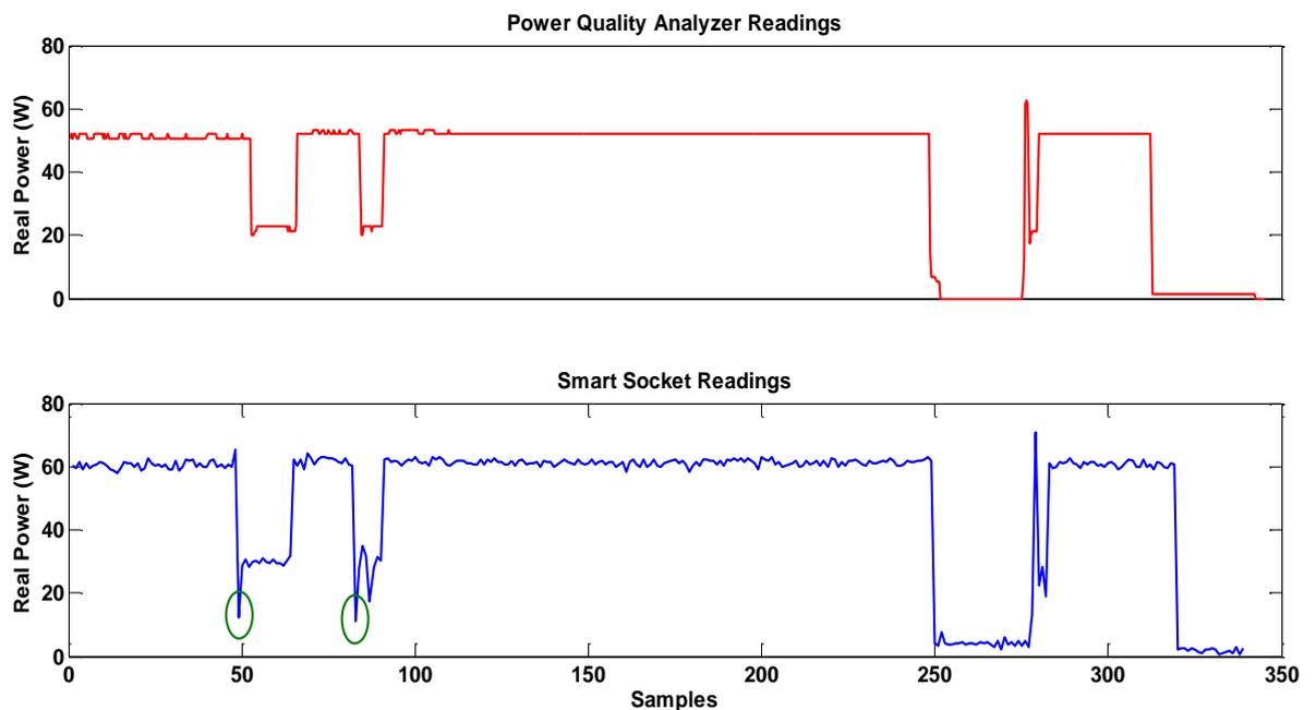
Figure 35: Power consumption trend of LED TV as monitored by smart socket and PQA
