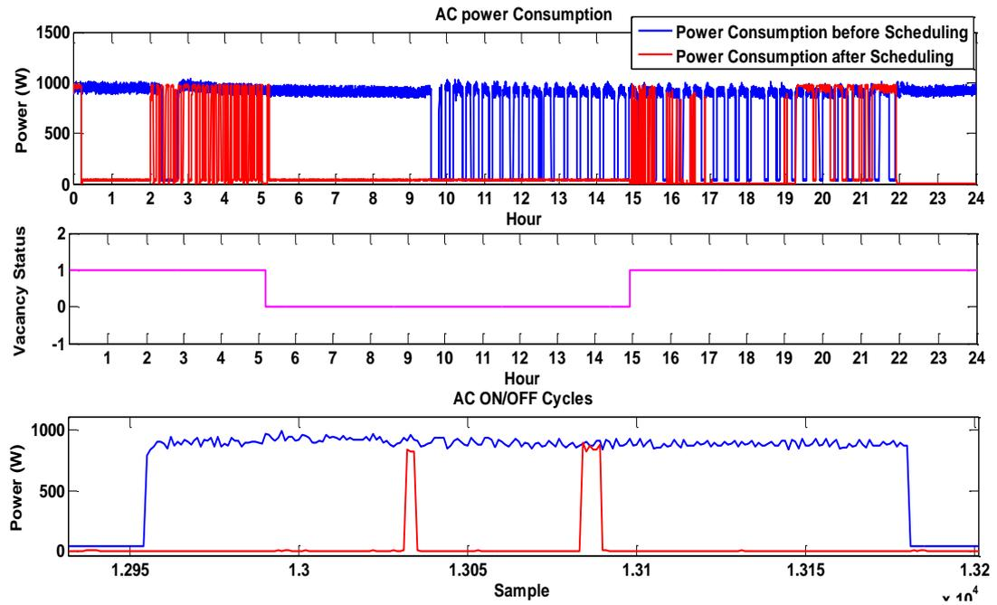
a) Power consumption trends of AC, room vacancy status, and on/off cycles of the AC before and after the application of the algorithm
