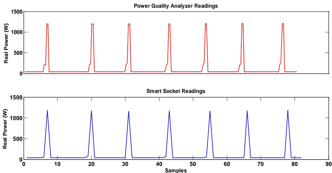
Figure 37 :Power consumption trend of microwave oven as monitored by smart socket and PQA
