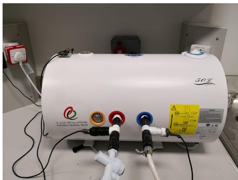
Figure 25: Experimental setup of the water heater
