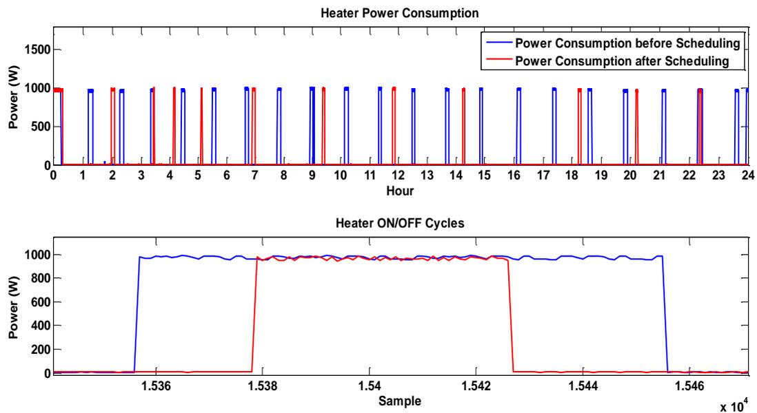
a) Power consumption trend of the heater before and after the application of the energy management process
