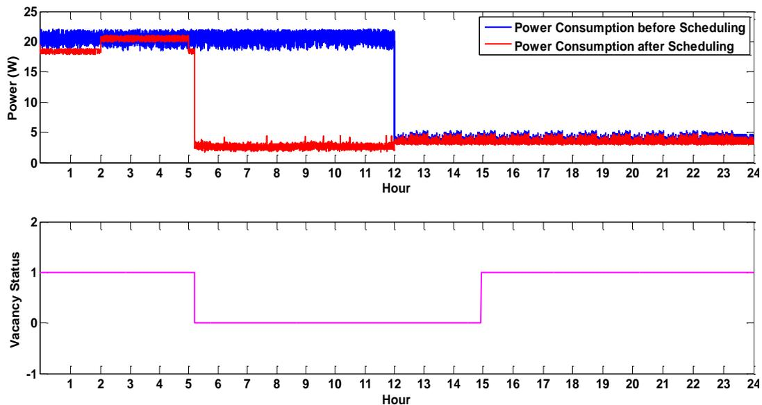
a) Power consumption trend of the LED light before and after the HEM process is utilized along with the vacancy information during the HEM process
