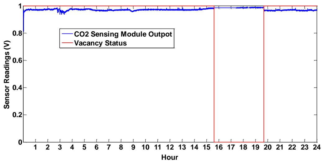
Figure 30: Relationship between CO<sub>2</sub> sensor readings and the occupancy status of the room (24 h monitoring period)
