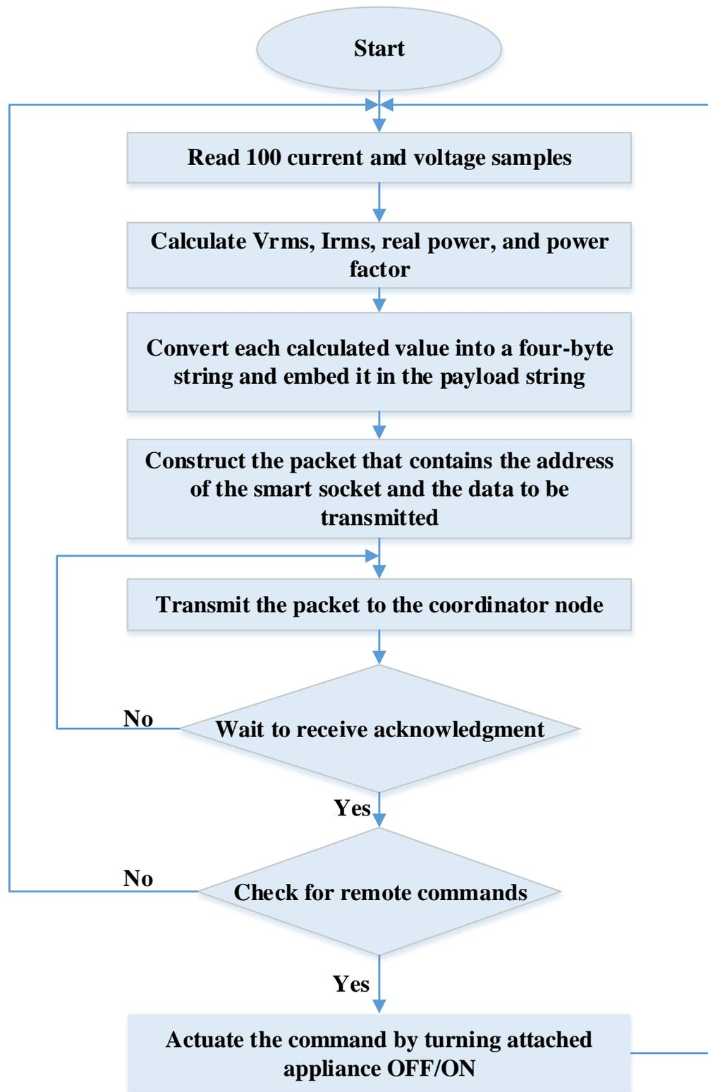
Figure 15: Smart socket data processing steps
