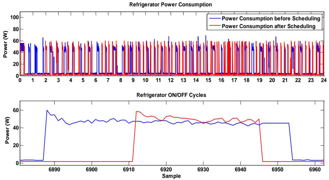
a) Power consumption trend of the refrigerator before and after the application of the energy management process
