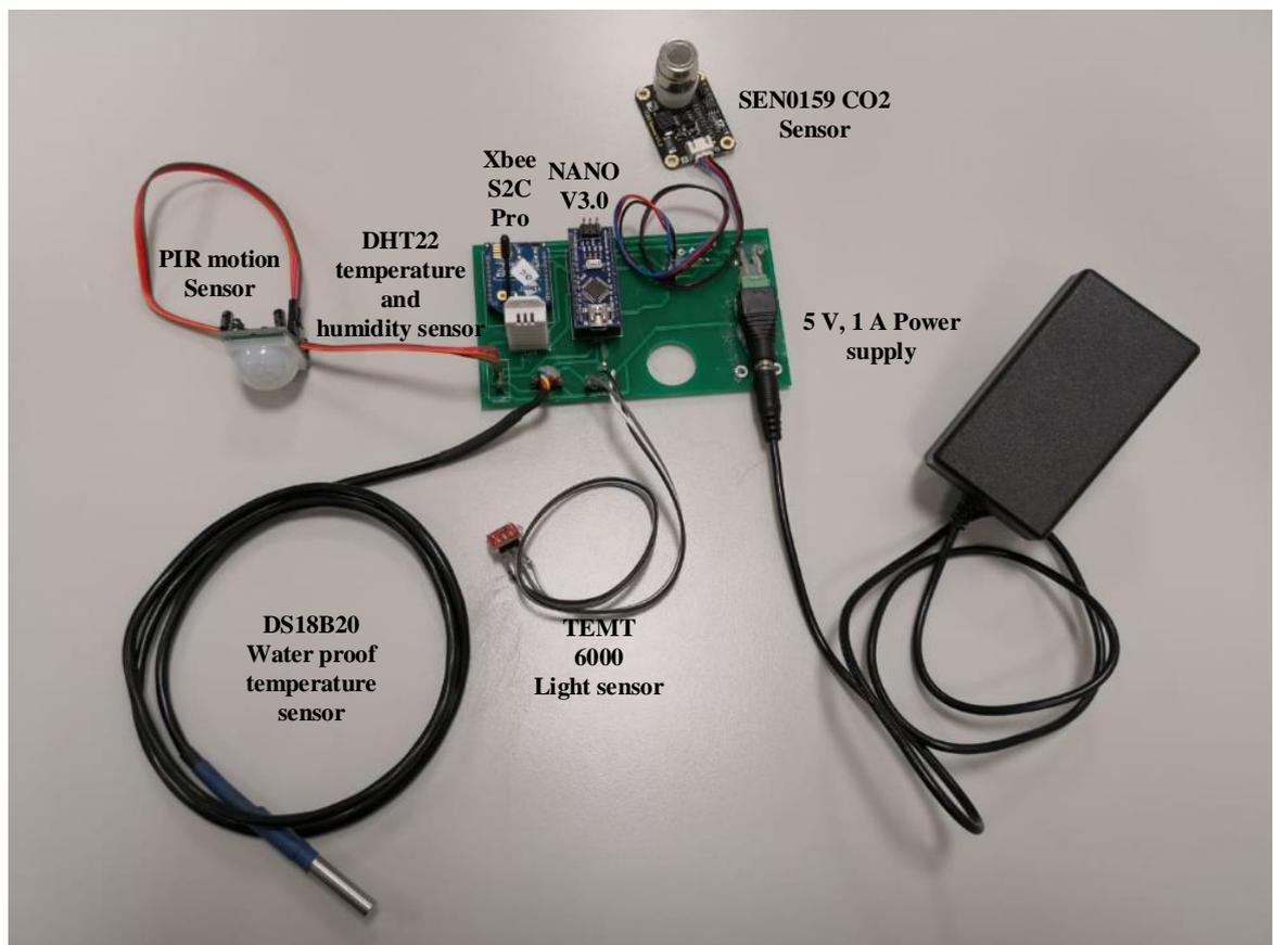
Figure 11: Room condition monitoring circuit
