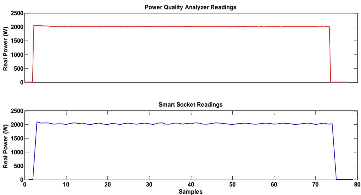
Figure 38: Power consumption trend of electric kettle as monitored by smart socket and PQA
